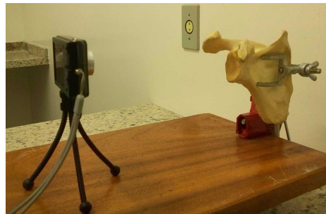
Fig. 1. Mounted system for capturing images related to the angles of the slope of the acromion and scapular spine.
