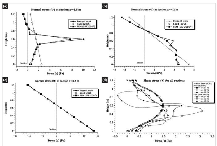
Figure 4 - Numerical and analytical results for example 2: (a) normal stress at x=4.6m; (b) normal stress at x=4.2m; (c) normal stress at x=2.4m; (d) shear stress for all sections.
