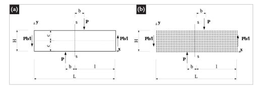
Figure 1 - Beam subjected to two equal forces P: (a) geometry; (b) model discretized in field nodes.
