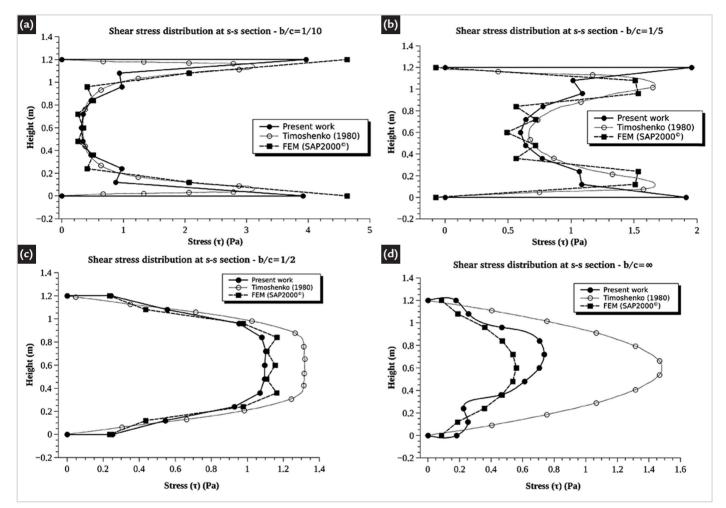
Figure 2 - Numerical and analytical shear stress for Example 1: (a) b/c=1/10; (b) b/c=1/2; (c) b/c=1/2; (d)  $b/c=\infty$ .
