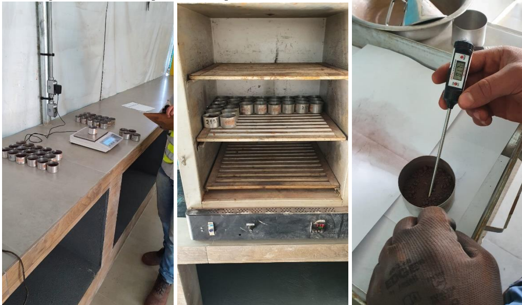
Figure 1— Standard procedure steps: mass definition, oven use and temperature check
