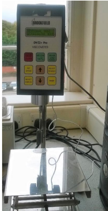
Figura 7.15: Viscosímetro Brookfield DV-II Pro (Institute of Particle Science and Engineering, Leeds University, 2014).
