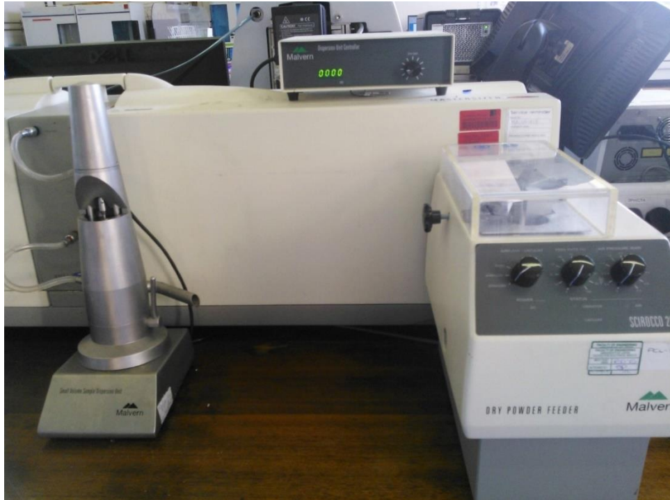
Figura 4.15: Analisador do tamanho de partículas, Malvern Mastersizer 2000, Malvern Instruments Ltd., UK (Institute of Particle Science and Engineering, Leeds University, 2014).
