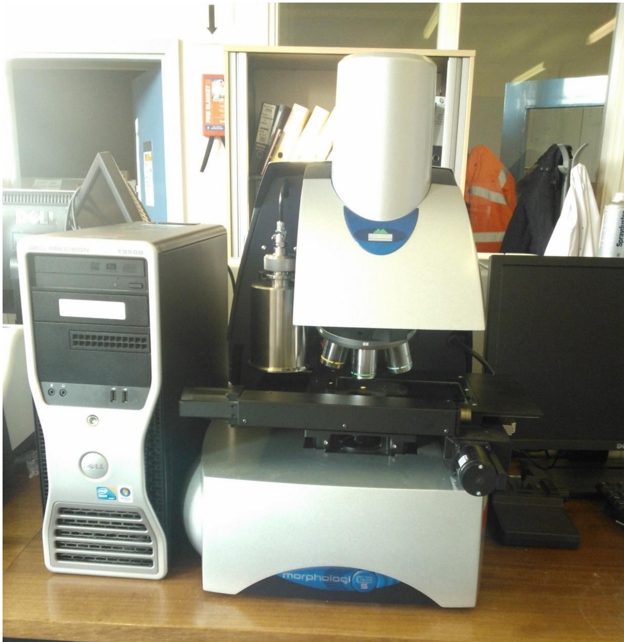
Figura 4.13: Automatizador de partículas Morphologi G3 (Institute of Particle Science and Engineering, Leeds University, 2014).
