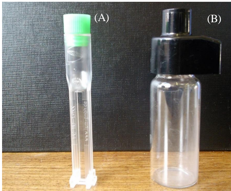
Figura 6.8: Destaque para as células de análise, em (A) Lumisizer e (B) Turbiscan. (Institute of Particle Science and Engineering, Leeds University, 2014).
