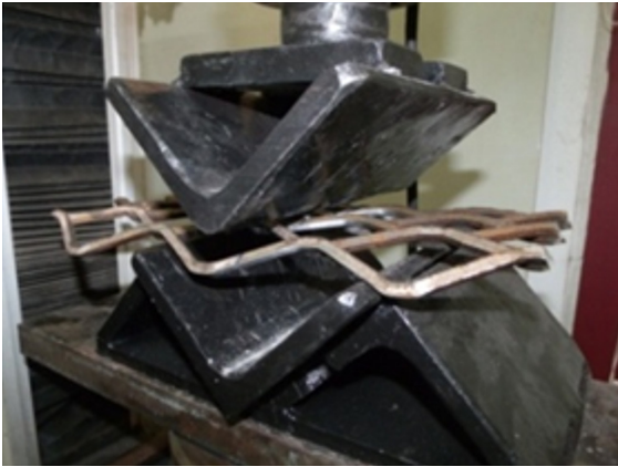
Figure 3. Developed device for bending test on extended sheets (90°).
