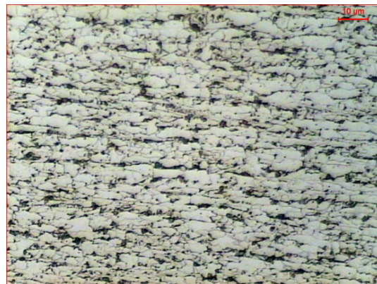
Fig. 3. Microstructure of the steel used in the control arm. (Nital 2%, OM 1000X).
