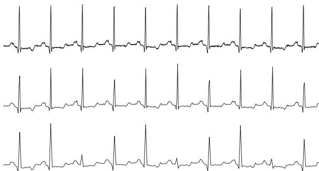
Fig. 1. ECG signal sampled in low frequencies. In the first row, it is shown the original ECG signal, while in the last two ones the corresponding signal sampled in 60 Hz and 30 Hz, respectively.
