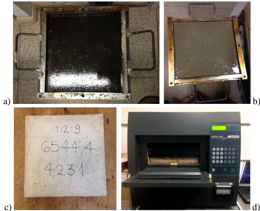
Figure 3-1 – Steps on the fabrication and testing of the boards: a) Mould prepared b) Mould filled with mortar c) Resulting mortar board and d) Testing on HFM equipment
