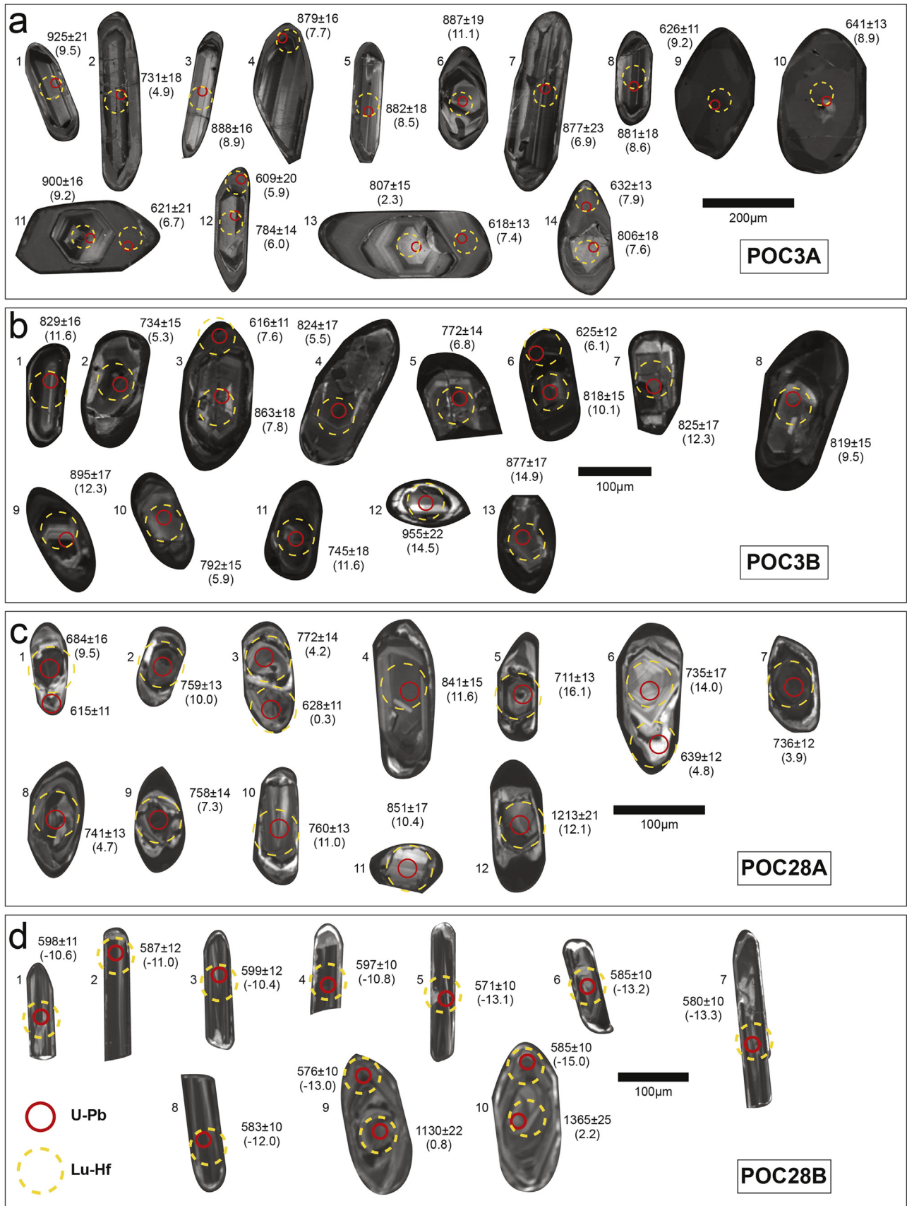
Figure 3. Representative CL images with U–Pb and Lu–Hf spots of analysed zircons. The U–Pb ages are reported in Ma as ^{206}\text{Pb}/^{238}\text{U} ages for zircons <1000 Ma and ^{207}\text{Pb}/^{206}\text{Pb} ages for zircons >1000 Ma with errors at the 2\sigma level. Calculated \epsilon_{\text{Hf}}(t) values are given in brackets.
